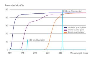
The discharge of low pressure lamps generally emits radiation at wavelengths of 185nm and 254nm. While all lamps made of the diverse material (natural, synthetic or doped quartz) have approximately the same output at 254nm, the output at 185nm depends on the quartz type used.
