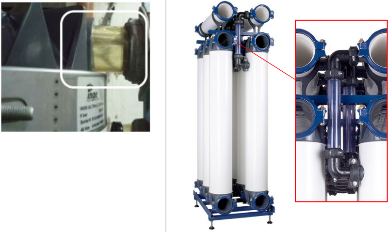
Figure 12.4-3 - Monitoring and ensuring error-free operation of the assembled rack with the help of an integrated transparent pipe on the feed side (in the PES-UF Modules for Open Platform - left) and on the filtrate side (in the T-Rack™ Series - right)
